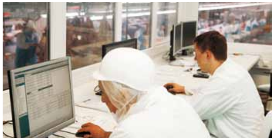
From the production control room it is possible to have an overview of the deboning hall system and at the same time monitor key performance indicators such as individual operator performance, yield and throughput.
